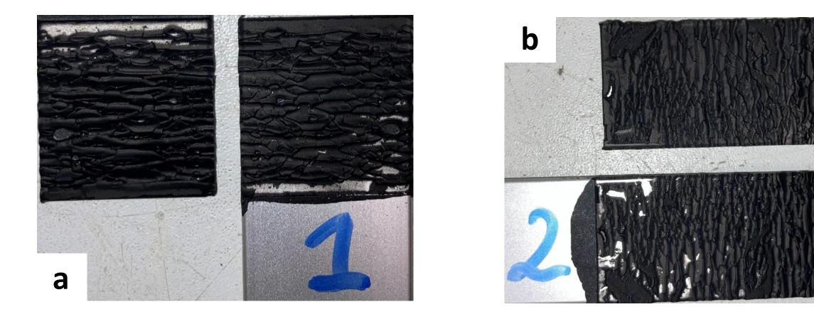
Figure 2 – Modes of failure: a) Al 25 [mm]; b) Al 50 [mm]
