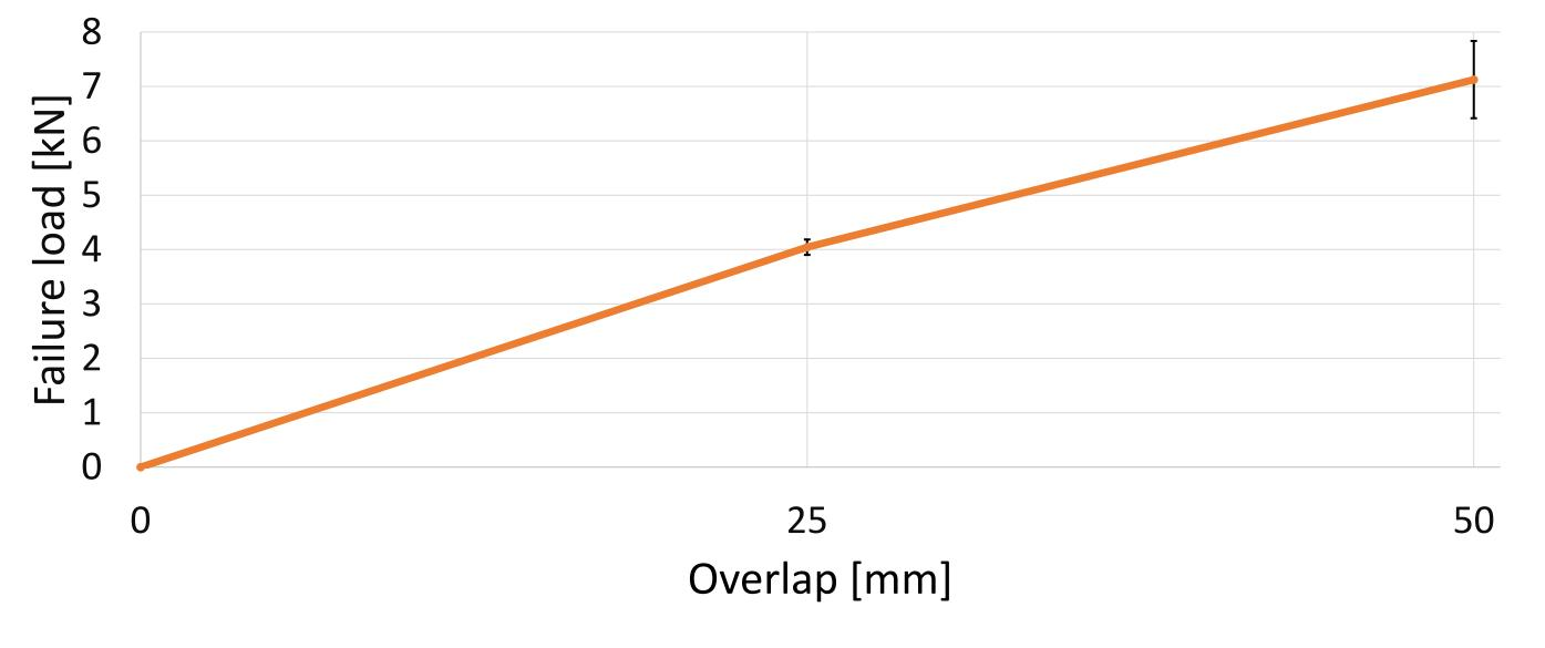
Figure 3 – Failure load vs overlap length for the aluminium SLJs
